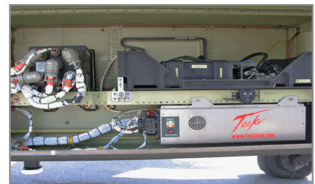
Replaces the original battery in the Apache 64D Helicopter.
