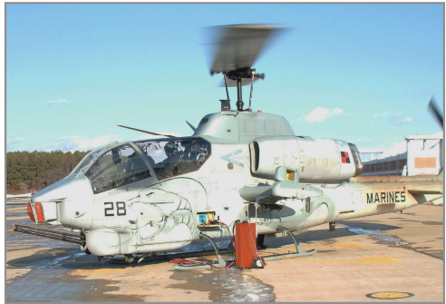
Currently being used with the Bell AH-1 Super Cobra. Designed for 24/48V simultaneous starts.
