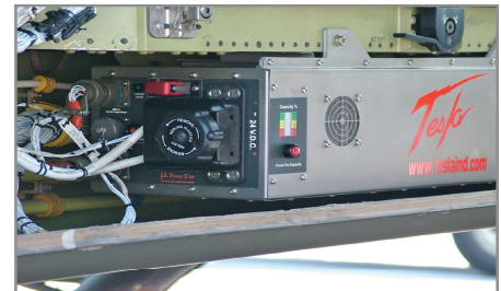
Replaces the original battery in the Apache 64D Helicopter.
